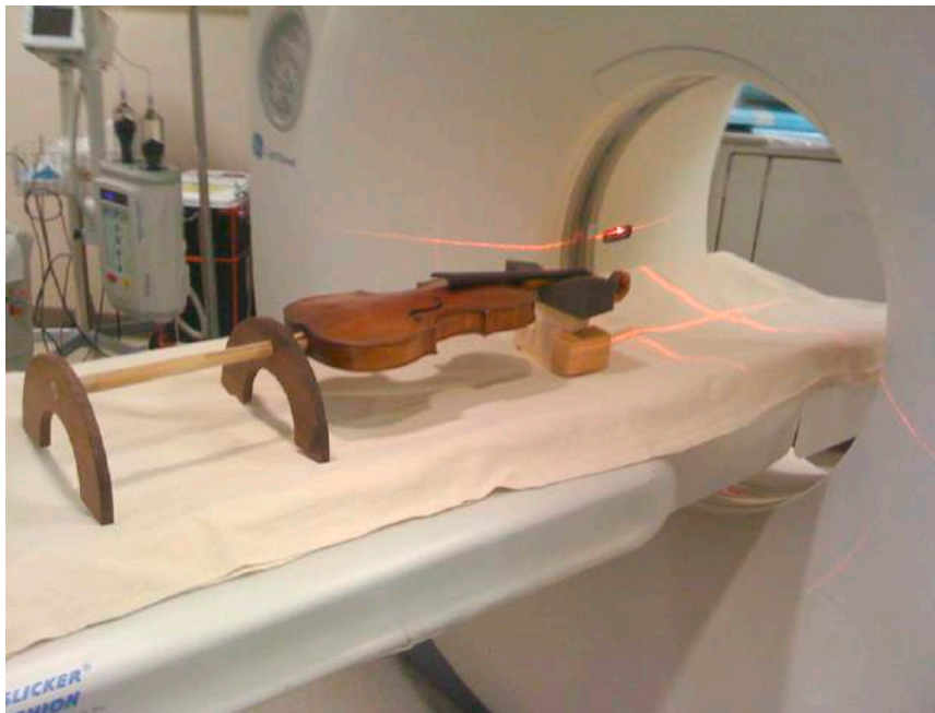
Figure 3. A violin in position for a CT scan measurement. A red He-Ne laser beam is used as the reference for positioning the axis of the violin with the x, y, and z-axes of the CT scanner. A special holding device attached to the end button elevates the violin above the table, facilitates alignment of the axis, and avoids artifacts from support material such as sponges.
